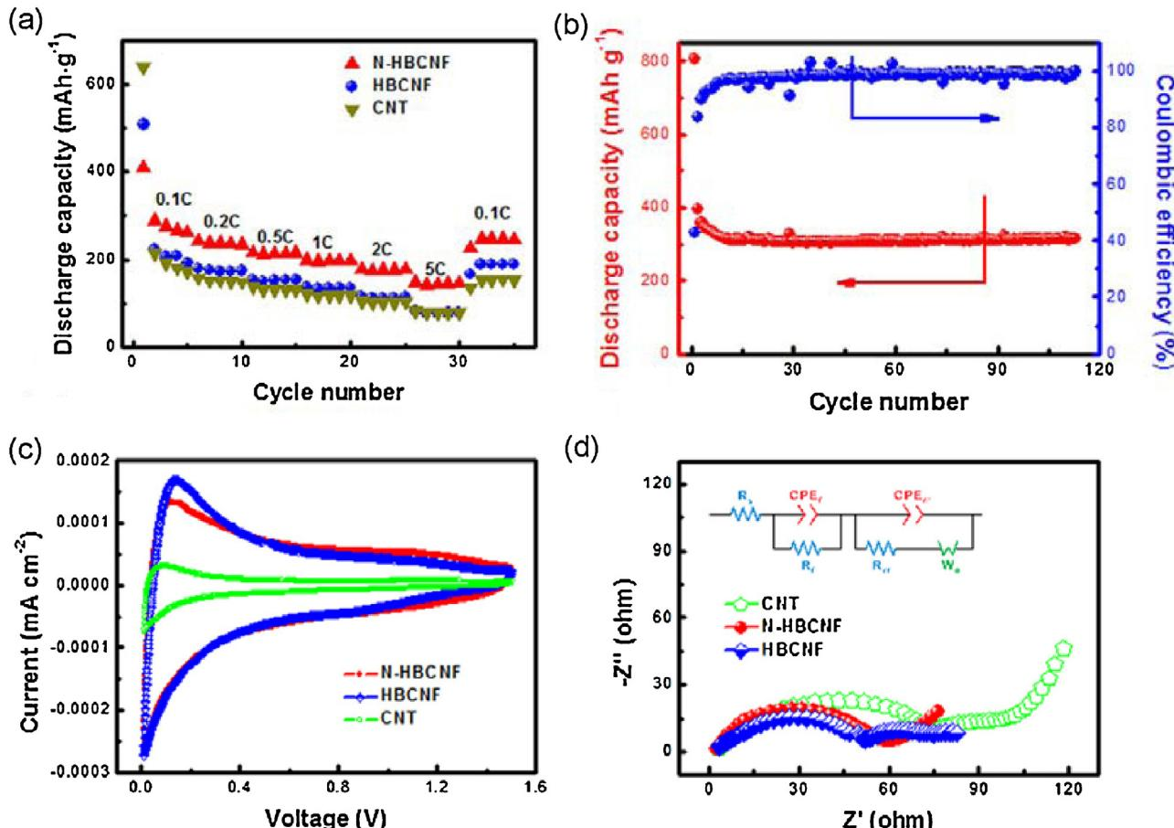
**Fig. 3.** Li ion storage performance of N-HBCNFs: (a) The charge/discharge performance of CNT, HBCNF, N-HBCNF anodes at different current densities (1.0 C = 372 mA g<sup>-1</sup>) and (b) the cyclic performance of N-HBCNF electrode with the current of 0.5 C, (c) the cyclic voltammetry curves of N-HBCNF, HBCNF, CNT anodes at a scan rate of 0.1 mV s<sup>-1</sup>, (d) the EIS spectra of CNT, HBCNF, N-HBCNF anode before cycles.
