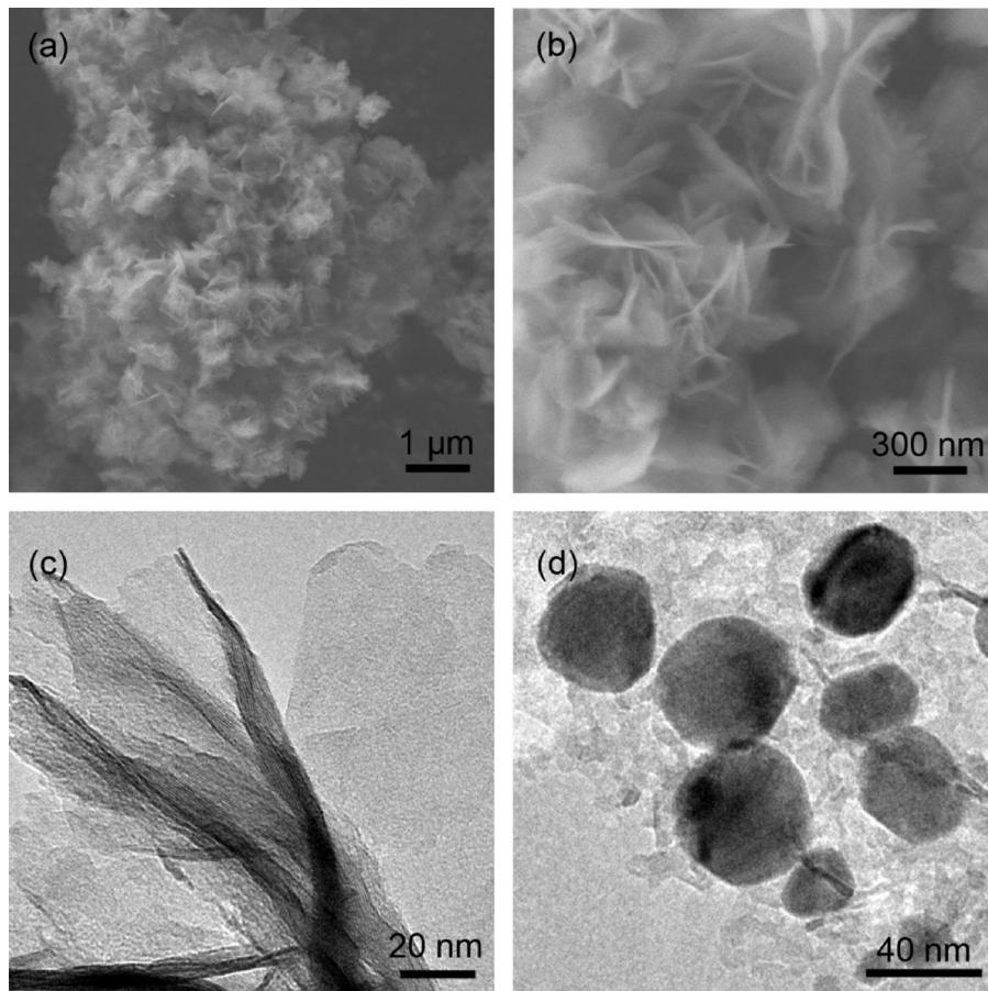
**Fig. 1.** LDH based catalysts for N-HBCNF formation: (a) The low and (b) high magnification SEM images of the NiAl LDH flakes; the TEM images of (c) LDH flakes and (d) reduced LDO catalysts for the N-HBCNF growth.
