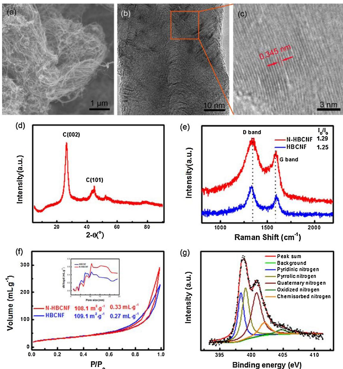
**Fig. 2.** The morphology and microstructures of N-HBCNFs: (a) SEM image, (b) low and (c) high magnification TEM images of N-HBCNFs; (d) The XRD pattern of the N-HBCNFs, (e) Raman spectra and (f)  $N_2$  isothermal adsorption and desorption curves of HBCNFs and N-HBCNFs, inset shows the corresponding pore size distribution, (g) XPS spectra in N region of the obtained N-HBCNFs.
