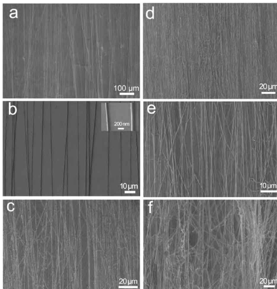
**Fig. 10.** The SEM images of well-aligned nanofibers collected by setup 2: (a, b) alignment after 10 s of spinning time (the inset in (b) shows enlarged SEM image of the nanofibers.); (c) after 30 s; (d, e) after 1 min; (f) after 2 min.
