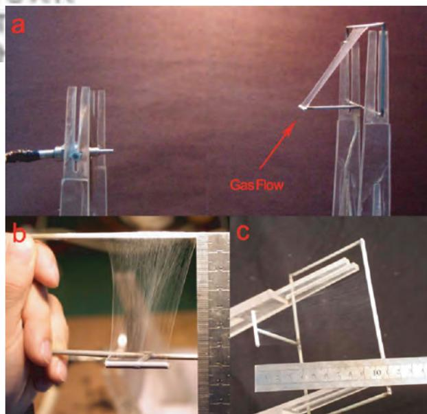
**Fig. 8.** (a) setup 2 for electrospinning; (b, c) the collector with the length of nanofibers over 10 cm.
