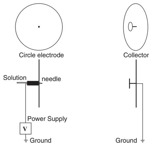
Fig. 1. The sketch of setup 1 for electrospinning.
