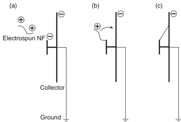
**Fig. 5.** The sketch of the orientation of the electrospun nanofiber on the collector of setup 1: (a) an electrospun nanofiber with positive charge is flying to the collector; (b) the front point of the electrospun nanofiber touches the smaller circle metal sheet and becomes a fixed site; (c) the end of the electrospun nanofiber flies to the bigger circle metal sheet.
