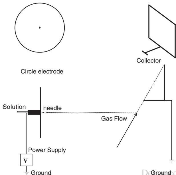
**Fig. 2.** The sketch of setup 2 for electrospinning.
