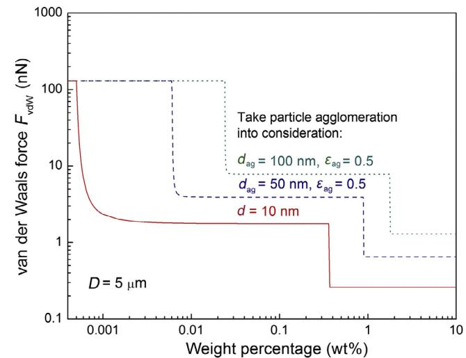
**Fig. 5.** Calculated van der Waals force against weight percentage of guest particles based on three-point contact model (where the dash lines further take the agglomeration of guest particles into consideration).
