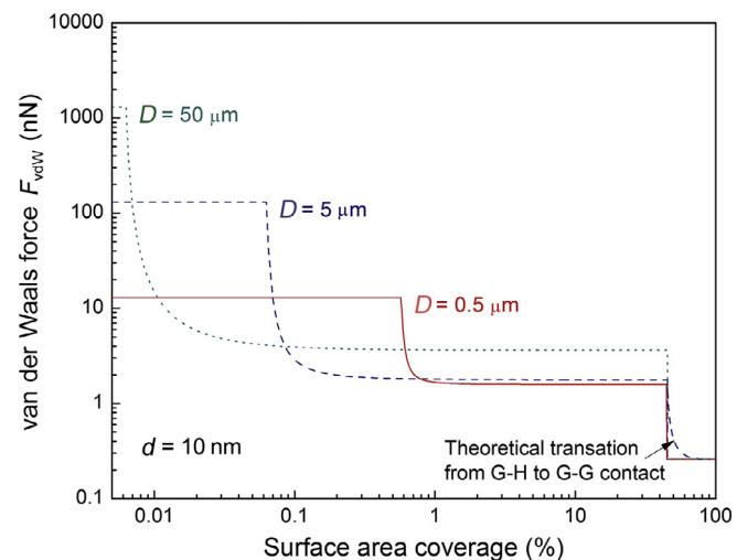
**Fig. 4.** Calculated van der Waals force against surface area coverage (SAC) based on three-point contact model (where the arrow points to the theoretical transition from guest–host to guest–guest contact which is omitted in this work).
