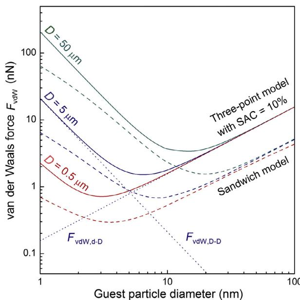
**Fig. 3.** Calculated van der Waals force against guest particle diameter based on three-point contact model (solid lines) and sandwich contact model (dash lines).
