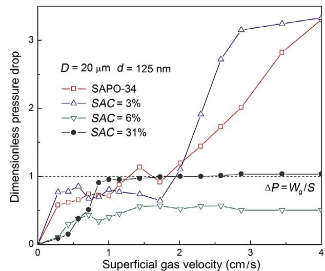
**Fig. 7.** Fluidization curves of coated SAPO-34 powders with different SACs.
