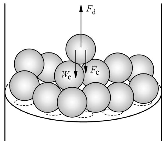
**Fig. 8.** Force analysis for a single particle in fluidized bed.
