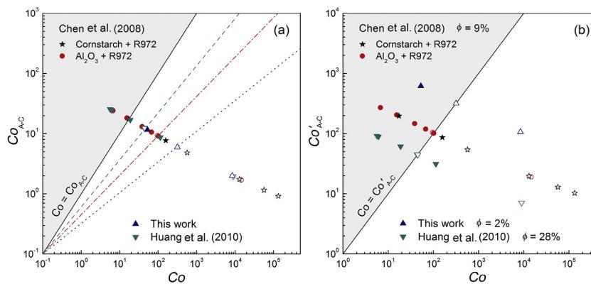
**Fig. 9.** Transition between Group A and Group C flow characteristics based on granular cohesive number before (a) and after (b) modification (where solid symbols indicate that the powders have been fully fluidized during experiment, and hollow symbols represent that the solids bed could not be fluidized entirely).
