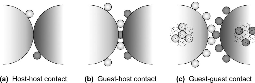
**Fig. 2.** Contact between two coated particles under different SACs (Chen et al., 2009).
