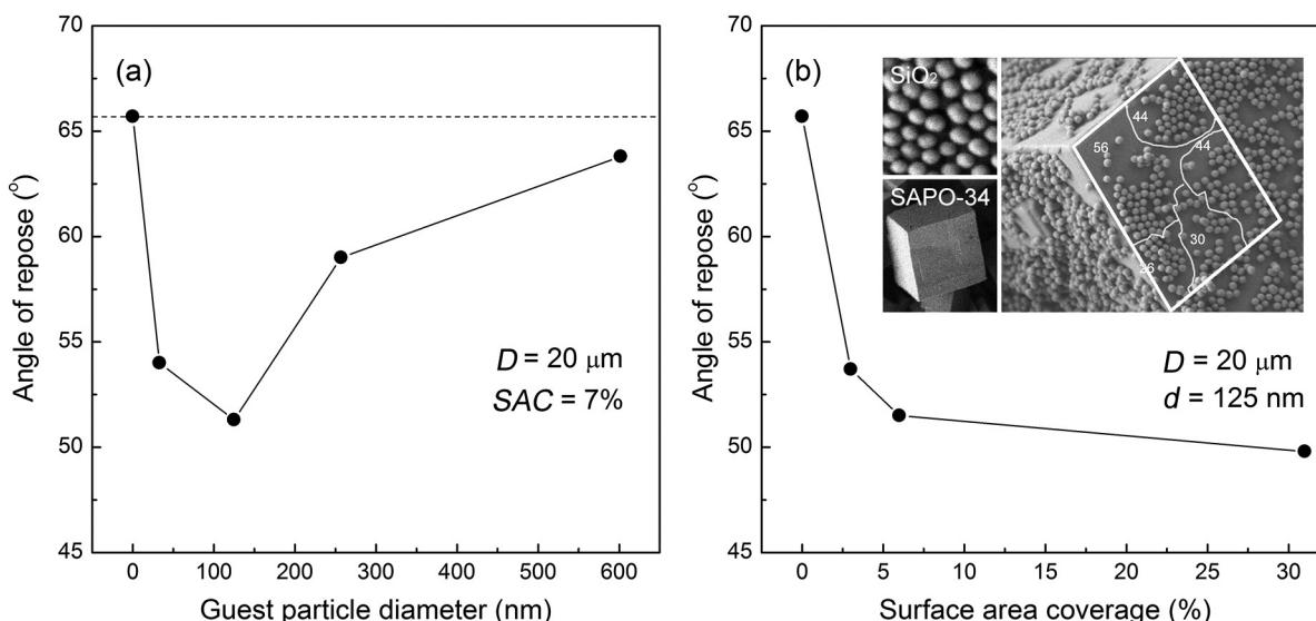
**Fig. 6.** Repose angles of coated SAPO-34 powders with various silica particle sizes (a) and surface area coverages (SACs) (b).
