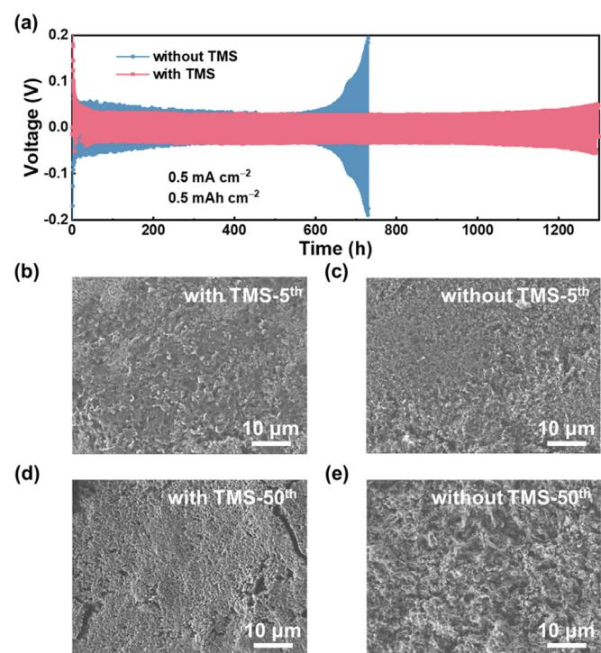
**Fig. 1.** Electrochemical performance of Li | Li symmetrical cells and SEM images of Li metal anodes after cycles with/without TMS additives. (a) Cycling performance of Li | Li symmetrical cells at 0.5  $\text{mA cm}^{-2}$  with a capacity of 0.5  $\text{mA h cm}^{-2}$ . The deposition morphology of Li at the 5<sup>th</sup> cycle with (b) and without (c) TMS additives and at the 50<sup>th</sup> cycle with (d) and without (e) TMS additives.
