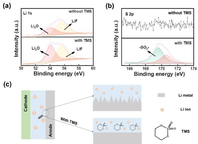
**Fig. 3.** XPS spectra of the SEI on ultrathin Li anode in Li | NCM523 batteries after 5 cycles. (a) Li 1s and (b) S 2p. (c) The schematics of the role of TMS additives in protecting ultrathin Li anode.
