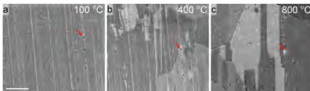
Figure 1. Surface modifications can be seen in snapshots taken during an annealing process at 100 °C (a), 400 °C (b), and 800 °C (c), respectively. A complete annealing process is shown in SI Movie M1. Red arrows reference identical positions on the foil. Sample movement is due to thermal drift. The scale bar measures 20 \mu\text{m} .
