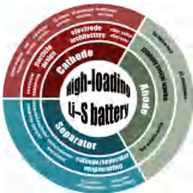
Figure 2. Schematic of the hierarchical design principle for high-loading Li-S battery.
