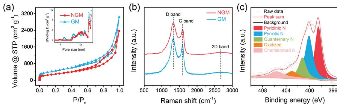
**Figure 2.** Structural characterization and properties of NGM materials. a)  $N_2$  sorption isotherms of NGM and GM, inset figure illustrates the pore size distribution. b) Raman spectra of NGM and GM. c) The high-resolution N 1s XPS spectrum of NGM.
