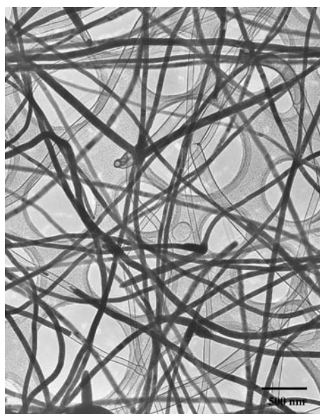
FIGURE 3 Detailed TEM image of large amount of Cu-filled CNTs and CNTs with totally hollow channel, without amorphous carbon on the outer wall
