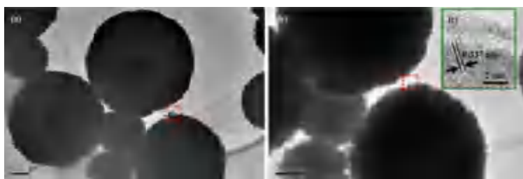
Fig. 4 Higher magnification TEM images (a, b) and HRTEM image (c) of the hydrothermally synthesized SrCO 3 submicron spheres deposited onto the holey carbon film, supported by a copper grid (molar ratio, additives: Na 2 CO 3 =5:100, SrCl 2 :Na 2 CO 3 =1.1:1, 190 °C, 12.0 h).
