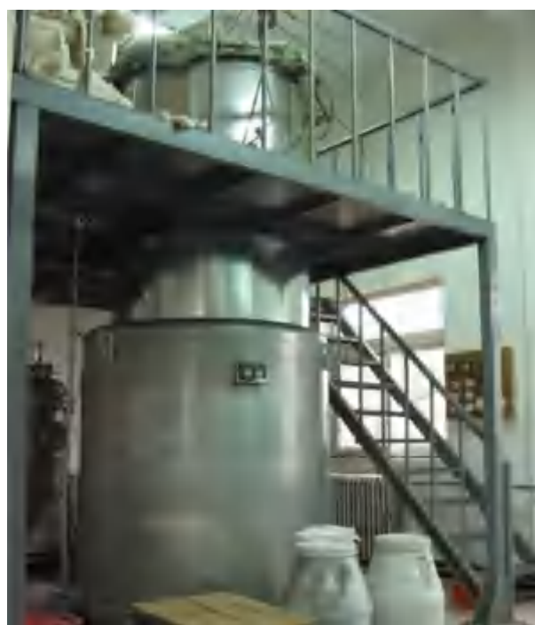
Fig. 13 – The pilot plant facility for VACNT array production at a rate of 3.0 kg/h.
