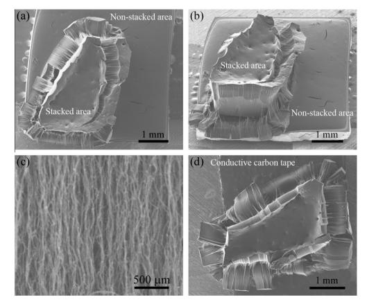
Fig. 3 – The SEM images of CNT arrays obtained on Substrate 1: (a) top view and (b) tilt view of the bottom substrate, the higher part corresponded to the stacked area; (c) alignment of CNTs in the millimeter-tall CNT arrays; (d) the top view of the CNTs grown on the cap substrate.
