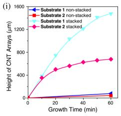
Fig. 2 – (a)–(h) The in situ recorded images for the growth of aligned CNTs on Substrate 1 (left part) and Substrate 2 (right part). (i) Growth curves of CNT arrays with and without the stacked of the cap substrates.
