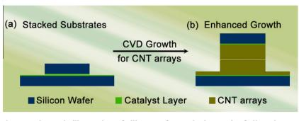
Fig. 1 - Schematic illustration of silicon wafer stacked growth of aligned CNTs.
