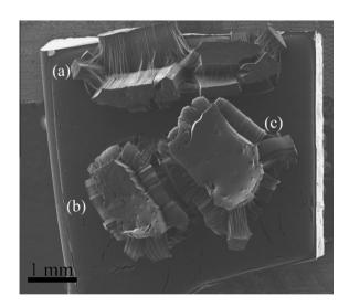
Fig. 5 – The morphology of as-grown CNT arrays on the substrate (silicon wafer with 3-nm-thick Fe catalyst film) by substrate stacking: (a) Si/SiO<sub>2</sub> wafer; (b) Si/SiO<sub>2</sub> wafer with Fe catalyst film; (c) 1-mm-thick quartz plate. In all cases, the CNT arrays grew faster in the stacked area of the substrates.
