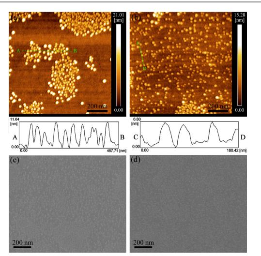
Fig. 6 – AFM topograph and height profiles of the catalyst surface after the annealing (a) in the non-stacked area of substrate and (b) in the stacked area; SEM images of catalysts after annealing in the (c) non-stacked area and (d) stacked area.
