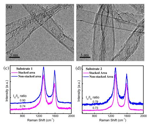
Fig. 4 – TEM images of CNTs obtained on Substrate 1 in (a) stacked area and (b) non-stacked area; Raman spectra of CNTs obtained on (c) Substrate 1 and (d) Substrate 2.
