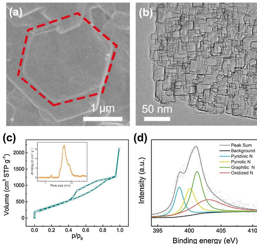
**Fig. 2.** Characterization of metal-free NMGF electrocatalyst. (a) SEM and (b) TEM images of NMGF. (c) Nitrogen adsorption–desorption isotherm of NMGF. STP is short for standard temperature and pressure. Inset: Pore distribution of NMGF. (d) High-resolution XPS spectrum of N 1s core levels in NMGF.
