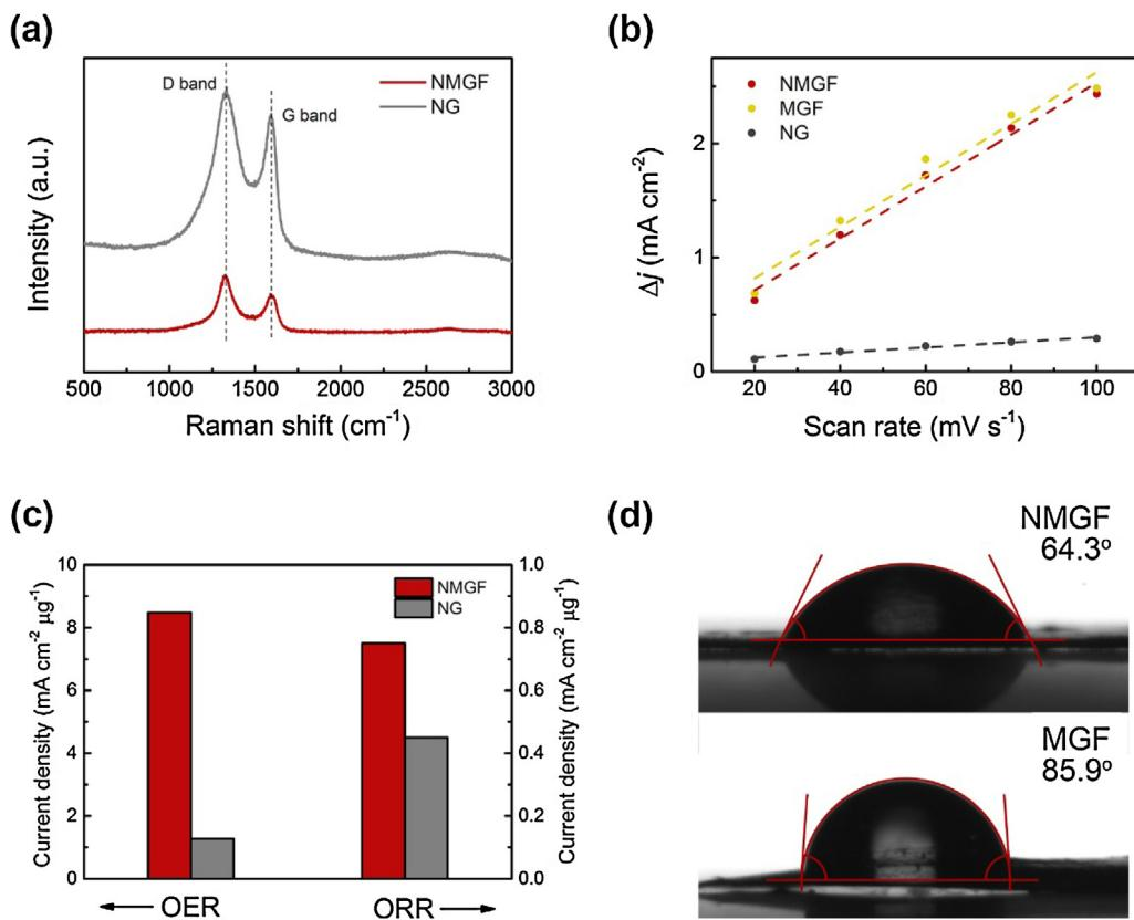
**Fig. 4.** The analysis of OER/ORR reactivity on NMGF electrocatalyst. (a) Raman spectra of NMGF and NG. (b) Charging current density differences plotted against scan rates. The linear slope, equivalent to twice the double-layer capacitance  $C_{dl}$ , was employed to represent the ECSA. (c) The specific current density of NMGF and NG based on nitrogen mass, tested at the potential of 1.80 V vs. RHE (OER) and 0.50 V vs. RHE (ORR). (d) The contact angles of NMGF and MGF.
