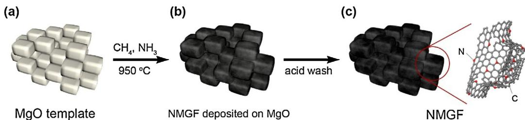
**Fig. 1.** The scheme of NMGF formation on porous MgO template.
