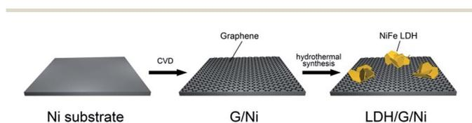
Scheme 1 Synthesis of LDH/G/Ni electrocatalysts with a graphene barrier between Ni substrates and layered NiFe hydroxides.
