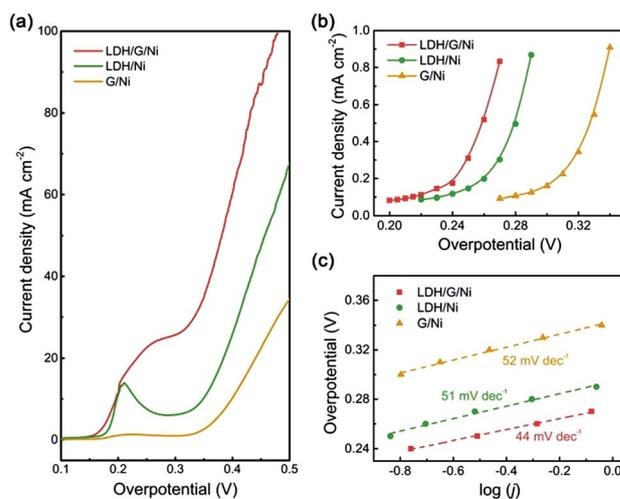
Fig. 2 OER performances of LDH/G/Ni electrocatalysts. (a)  $i$ - $R$  compensated LSV curves. The scan rate was  $10 \text{ mV s}^{-1}$ . (b) Voltammetric curves obtained by a chronoamperometric method. (c) Tafel plots. All the measurements were performed in  $\text{O}_2$  saturated 0.1 M KOH solution.
