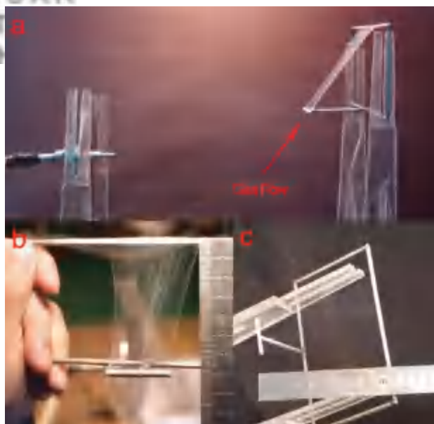
Fig. 8. (a) setup 2 for electrospinning; (b, c) the collector with the length of nanofibers over 10 cm.
