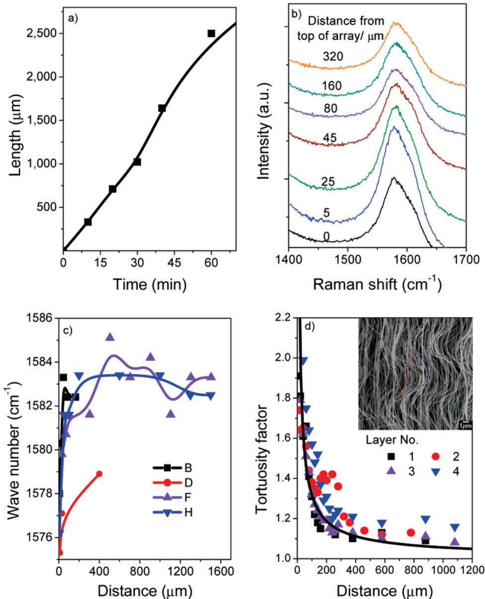
**Figure 2.** Quantitative description of the four-layer CNT array: (a) Growth rates in the floating catalyst process in the first hour, (b) Raman spectra of the first layer at different positions from the top, (c) Raman G band shift that corroborated the existence of stress in the array, and (d) tortuosity at different positions. The inset shows the measured tortuosity factor for the Type 2 (curved) CNTs defined as the length ratio of the blue to red lines.
